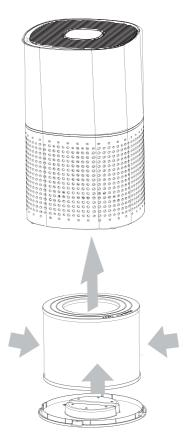
Polluted air enters through the air intake and is pushed through the filter which removes pollutants and flows through the air output on top of the purifier.
