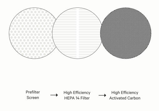
High efficiency HEPA 14 & activated carbon are combined in the same filter.
